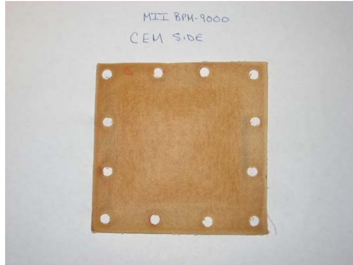
Figure 5.15 Used MII BPM-9000 Bi-Polar Membrane, CEM Side
