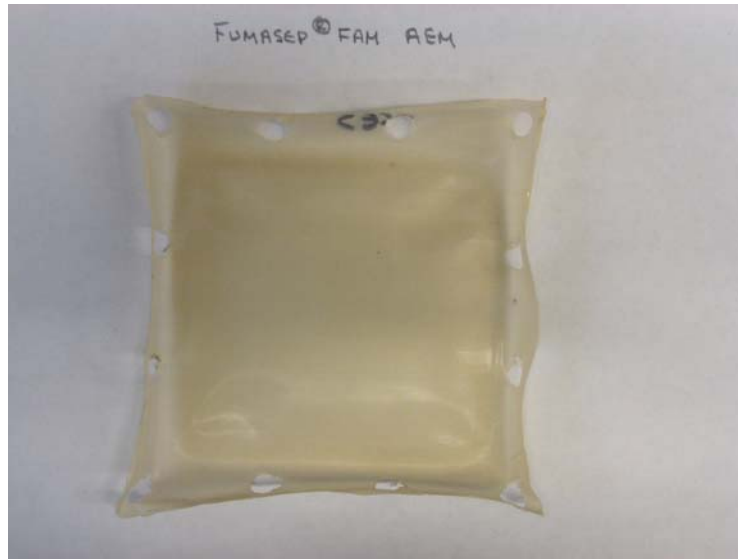
Figure 5.18 Used Fumasep® FBM Bi-Polar Membrane, AEM Side
