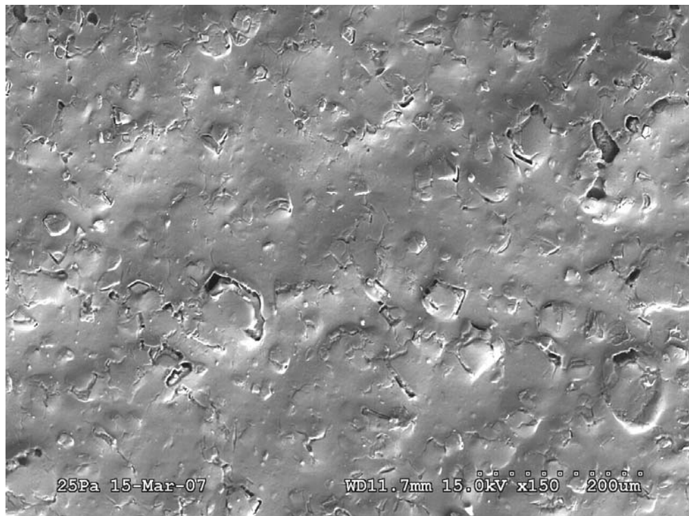
Figure 5.23 Used MII BPM-9000 SEM Image, CEM Side
