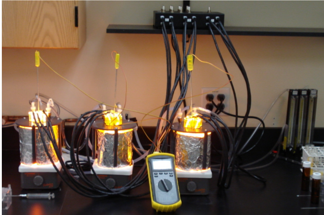
Figure 45 Photocatalytic Batch Reactors for SSS and VSSS Irradiation Experiments
