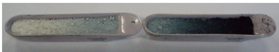
Figure 63 Thermochemically Ammonia Treated Degussa P-25 TiO 2 at 675°C at 87.3 mL/min. for 3 Hours
