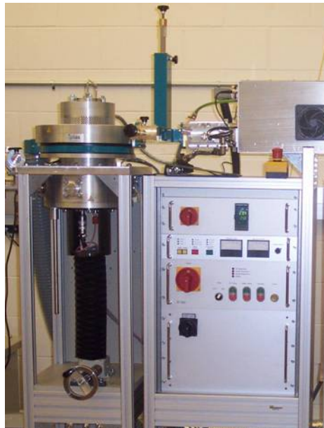
Figure 3.9: The Cyrannus I Iplas system used for deposition of NCD films.
