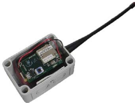
Figure 2: A Wireless Sensor Node for Flash-flood Alerting: Castillo-Effen et al., 2004, [7]
