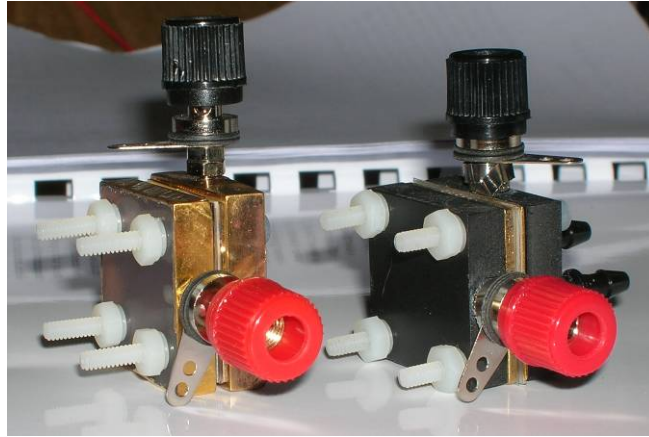
Figure 7.7. Prototypes of the single cell fuel cell stacks [98]
