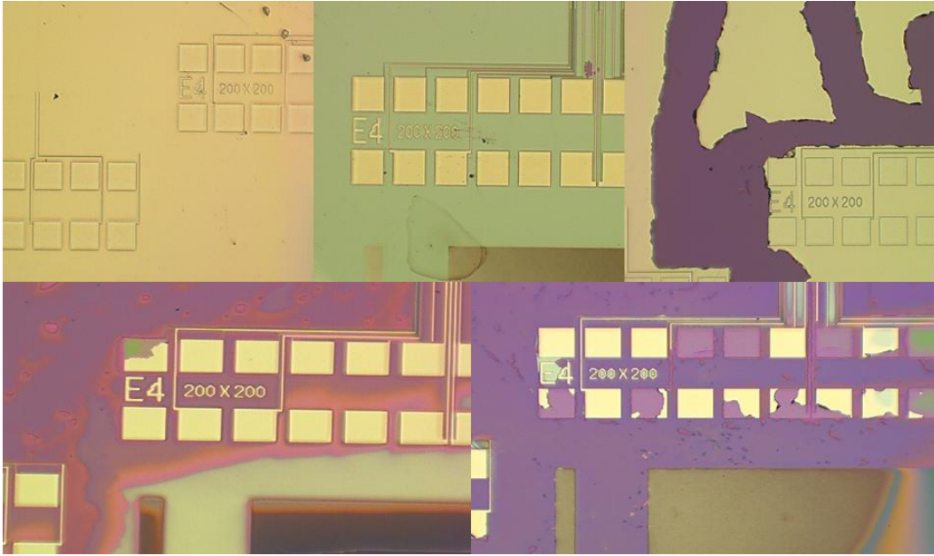
Figure 4.30 Pictures Showing Peeling on Wafers Polished at Different Temperatures. A) Wafer Polished at 15 °C. B) Wafer Polished at 20 °C. C) Wafer Polished at 25 °C. D) Wafer Polished at 30 °C. E) Wafer Polished at 35 °C
