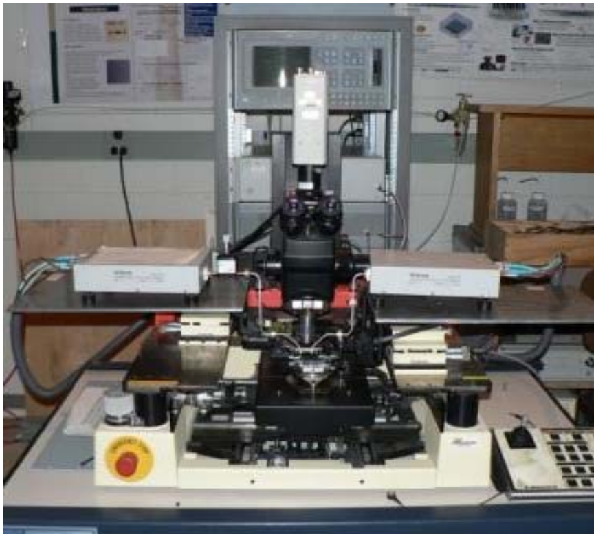
Figure C.1: Visual of the W band Measurement Setup.
