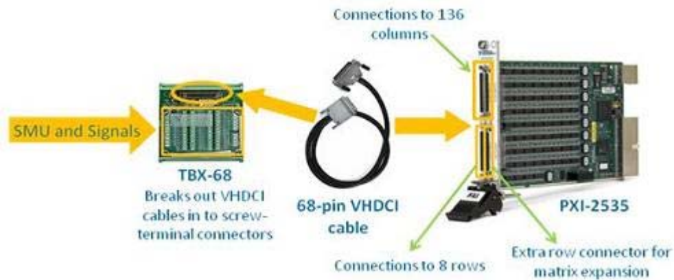
Figure 15: Connecting Signals to the PXI-2535
