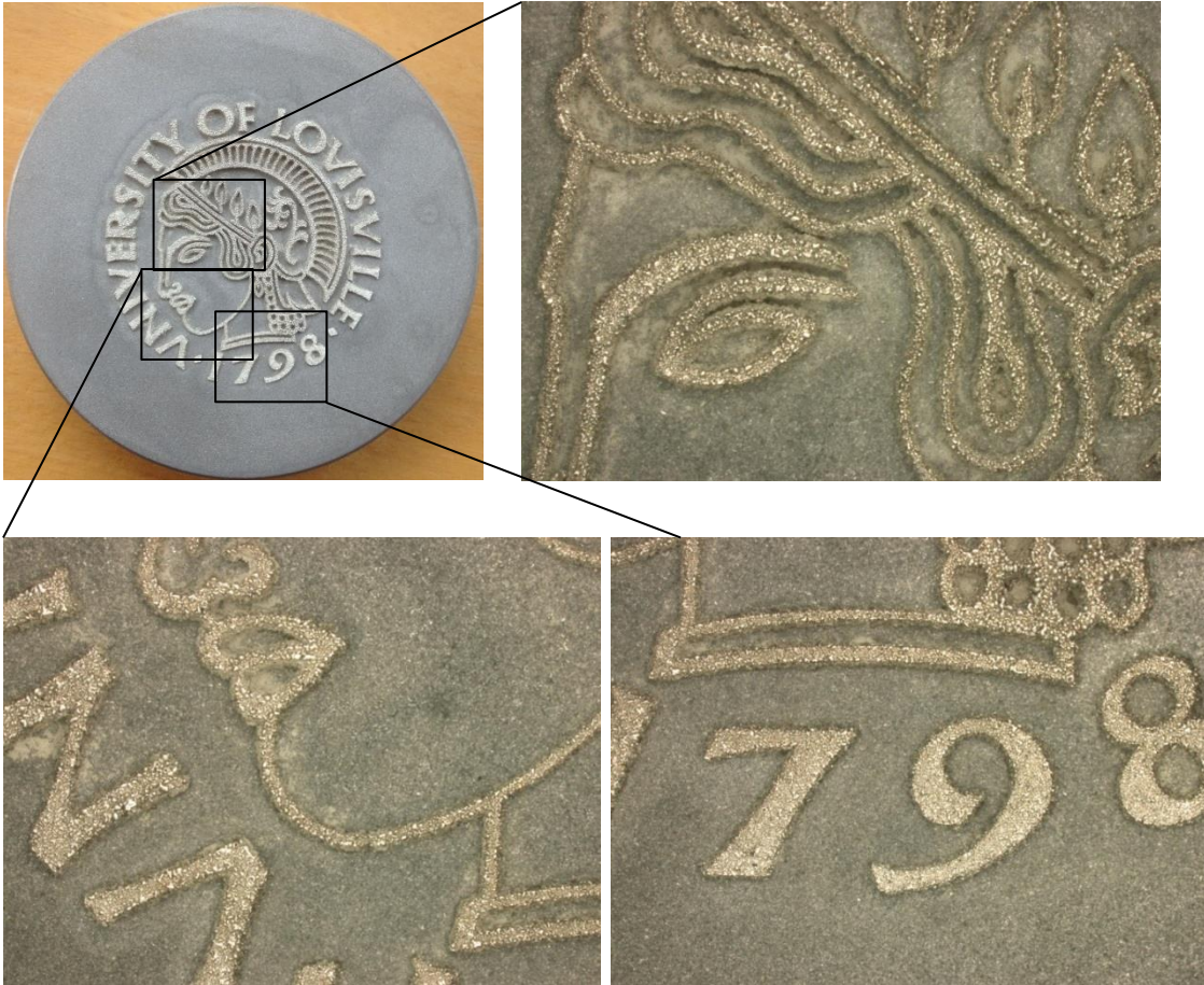
Figure 100: Manufactured University of Louisville Minerva batch a) as printed b) eyes 20 x magnification c) and d) details 20 x magnification
