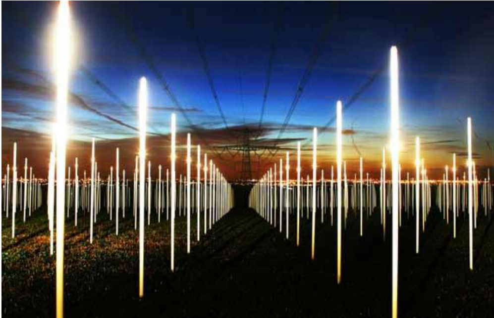
Fig. 1-4 Fluorescent tubes lit by EM field surrounding power lines
