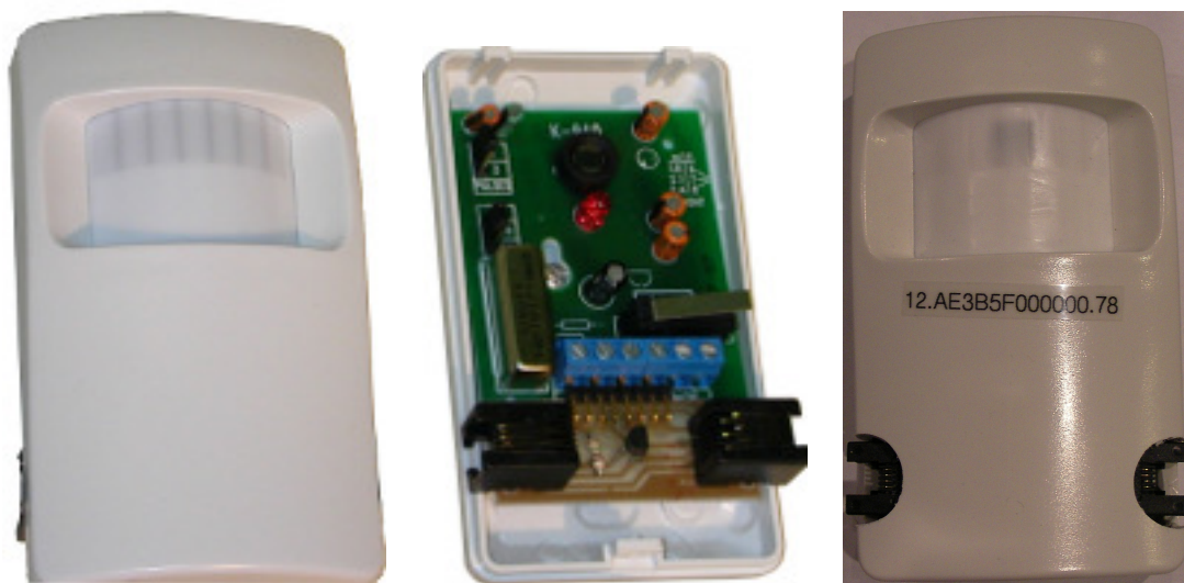
(a) A PIR area motion detector.
