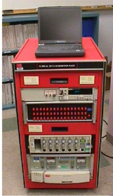
FIGURE 22 – DAQ system used to collect and store data from the mock flow loop studies used to characterize the cannula (30).
