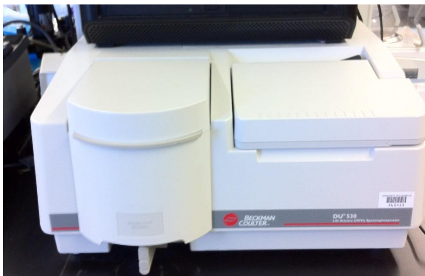
FIGURE 3—Spectrophotometer used for absorbance measurements.
