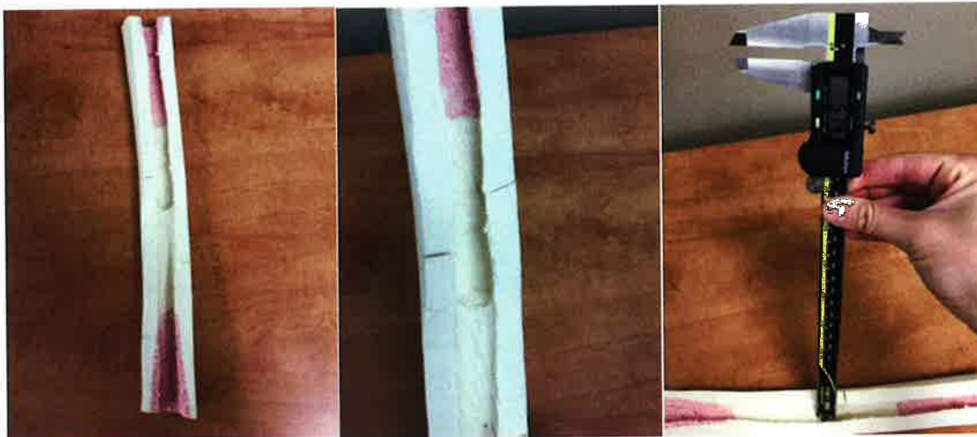
Figure 21: (Left) The second sawbones trial is shown above. The epiphyses were removed for this round of testing to allow the operator to more easily gage the distance of the reamer head down the IM canal of the sawbone. (Middle) A close-up view of the deflected cut is shown in the coronal plane. The sawbone experienced minor cracking during the cutting along the coronal plane to expose the deflected cut. This had no effect on the measured results of the experiment. (Right) The depth of maximum deflection was 5.74mm. No walking or otherwise detrimental effects of deflecting the reamer head are evident from the results meaning a successful experiment. From these results, the directional reaming system was proposed to be tested in a cadaver study.
