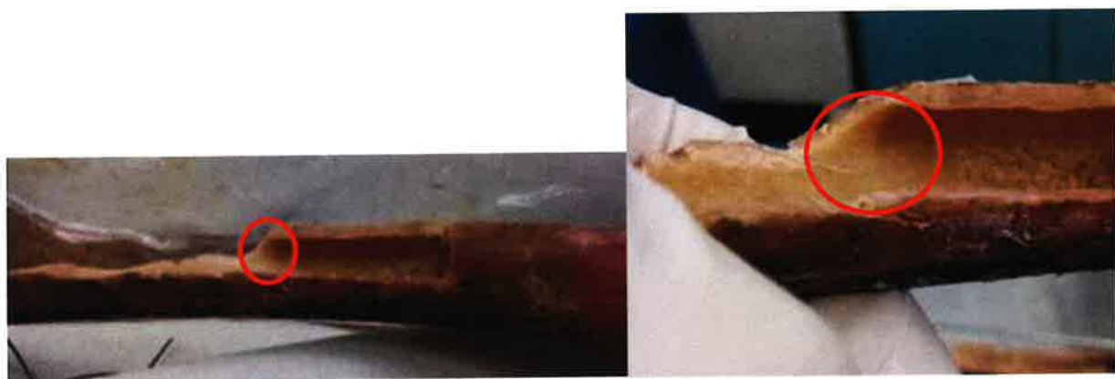
Figure 27: (Left) The second round of deflected reaming took place in the circled area shown above. The cut was made in the distal region of the femoral diaphysis on the medial wall. The deflected cut was exposed using an oscillating bone saw to create a quarter length cut along the diaphysis. (Right) A close up image of the deflected cut is shown in the darker shaded side of the image. The deflected cut is called out in red.
