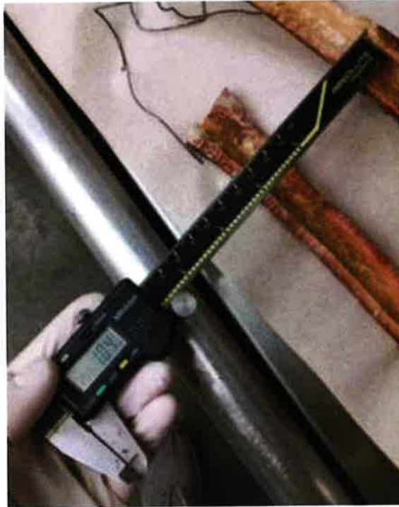
Figure 28: The maximum amount of deflection at this location was found to be 1.04mm. Thus, this model of a directional reaming device did not achieve the qualifying criterion of 3mm of lateral deflection as dictated in the experiment objectives. The main contributing factor to this result is bearing wear due to the friction between the stainless steel follower sleeve and the peek bearing. A possible solution to this issue is reversing the materials of the follower sleeve and bearing. However, a more practical solution may be found with the next iteration of the directional reaming system involving a canal plug and reamer shaft saddle.
