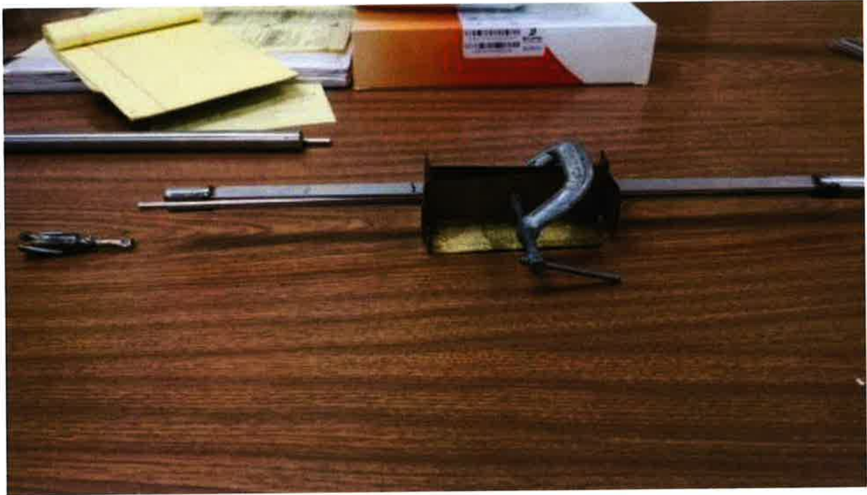
Figure 31: The third prototype exhibiting the separated reamer shaft is shown above. It is hypothesized that the washer used to prevent the weld from binding within the plug impinged on the inner wall of the canal. The shaft failed on the outer edge of the cortical model possibly indicating a bending moment was created between the edge of the stainless steel plug and the distal edge of the reamer head. The added distance from the weld and the shim would have increased the bending moment on the shaft as the plunger was driven into the plug. The plates held onto the attachment arms were included only to maintain alignment of the plunger and shaft within the attachment arms during operation.
