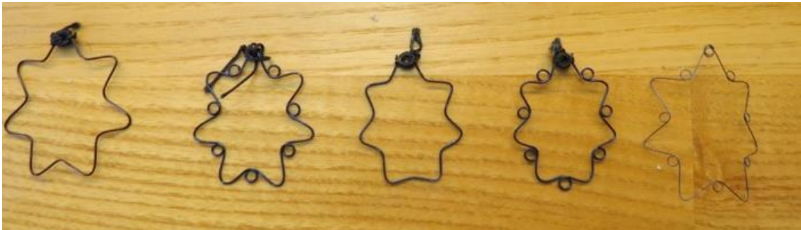
Figure 18: Photograph of candidate prototype nitinol connectors of various wire gauges, curved/flat members, and with/without loops.
