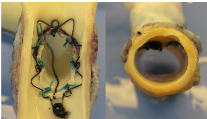
Figure 19: Photographs of 0.36 mm gauge nitinol connector providing smooth conformation to the luminal wall of a bovine descending aorta specimen.
