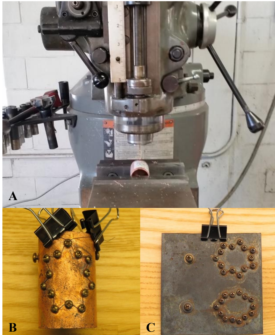
Figure 17: Photographs of the nitinol connector frame fabrication. A) Mill used for boring holes according to template mounted onto copper slip coupling, B) Copper slip coupling used to create curved nitinol connectors, C) Steel plate used to create flat nitinol connectors.
