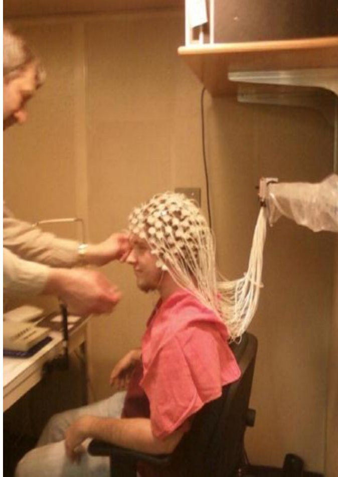
Figure 2 - The 128-channel EEG sensor net and testing room used in this study. The net was adjusted to fit the scalp of each subject individually to ensure that the electrodes were appropriately placed. The subject was seated in front of a computer display where visual stimuli were presented for the categorization task. Note that the subject seen in this picture was not a participant of this study.
