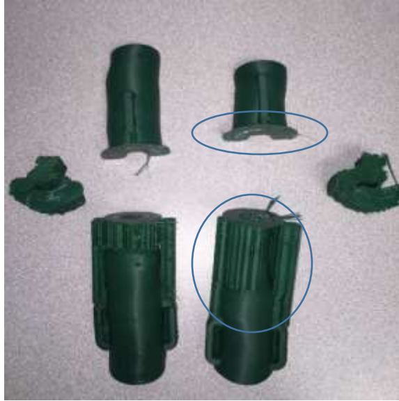
FIGURE 48- Prosthetic Devices After 3d Printing.
