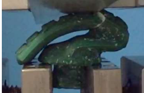
FIGURE 68- Ultimate Failure Of The Prosthetic Device.
