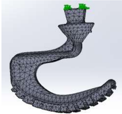
FIGURE 26- Beta Prototype Design Fixed Geometry And Finite Element Mesh In Static Simulation.
