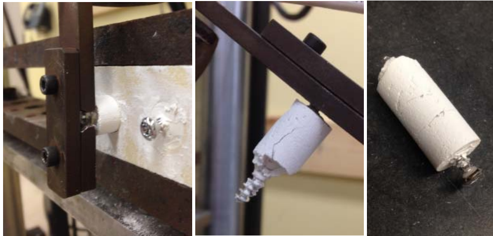
Figure 70: In the case of high density calcium phosphate 12mm hole samples, the inherent nature of the CaP cement to cure to the shape of the container caused the cement samples to slide directly out of the smooth cylindrical voids of the high density foam blocks when subjected to direct pullout forces. The left and middle picture shown above depict a sample with the locking plate attached as this combination often provided the more intact CaP cylinders at the end, although the same phenomenon occurred with the nonlocking plate attached.
