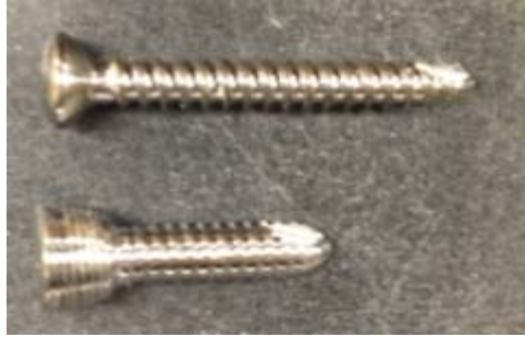
Figure 11: A visualization of the difference between locking head screws (bottom) and traditional smooth head screws (top). The locking head screws have threads along the head which is thicker than the alternative, and it transitions directly to the body without a “neck” region. This design increases the strength throughout the locking screw and allows the plate to hold it in a “locked” 90 degree angle.
