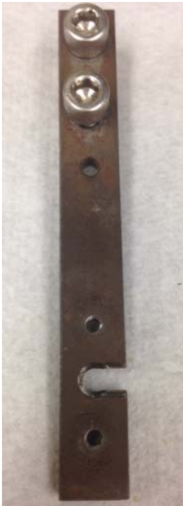
Figure 3: Up close view of the Custom plate. Screw heads fit in the slot towards the bottom and a Locking or Non-locking attachment was then secured around the head of the screw to simulate the correct screw head type.
