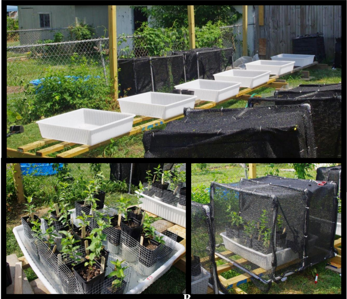
Figure 3-2. Outdoor mesocosm construction. A. The six experimental tanks arranged on a level, wooden riser. B. Seedlings arranged within a single experimental tank, without surrounding shade cloth enclosure. Metal crates on each side of the tank (three per side) correspond to the three different flooding durations, each containing four seedlings (one of each flooding depth). C. A completed mesocosm with a shade cloth enclosure. Each shade cloth enclosure bisected the tank into two light treatments (30% and 80% shade).
