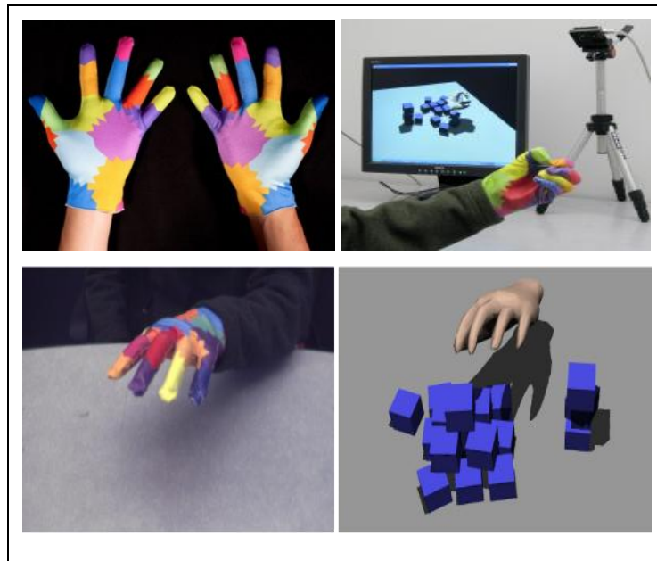
Figure 3.6: Colored gloves used for hand detection and tracking [37].
