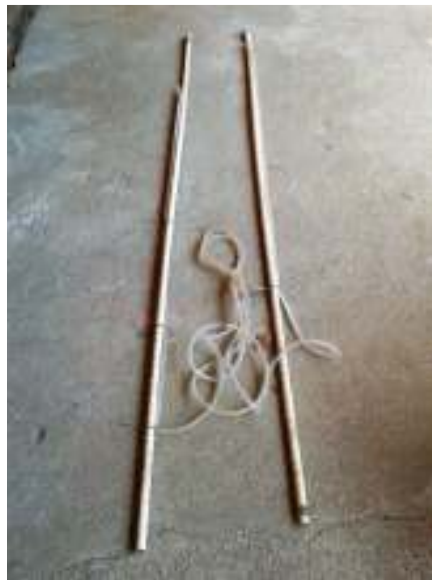
Figure 7: A Completed Water Level
