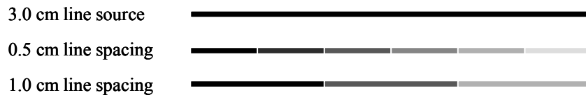
Figure 2-5 LSS approximation for a 3.0 cm length, using spacing of 0.5 cm and 1.0 cm.
