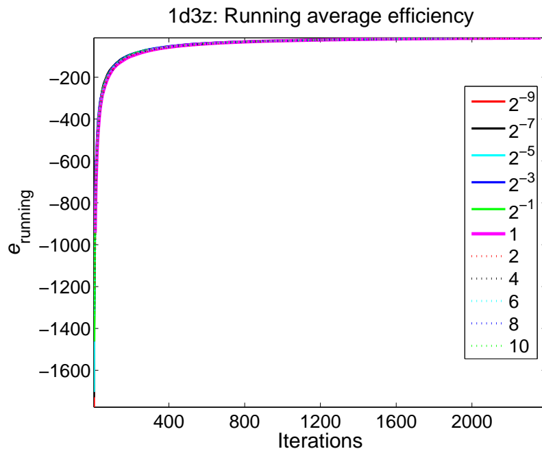
Figure 5.84: The running average efficiency, e_{\text{running}} , versus iterations for protein 1d3z with various values of n . Lower values mean better running average efficiency.
