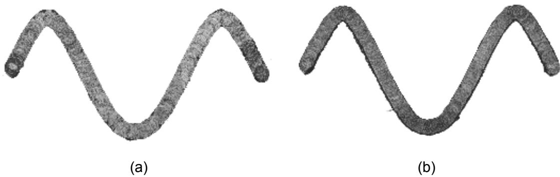
Figure 5.12: Images of cut sine wave pattern after background image removal for Test 4, Trial 1 for (a) EVF-NURBS and (b) VFIS
