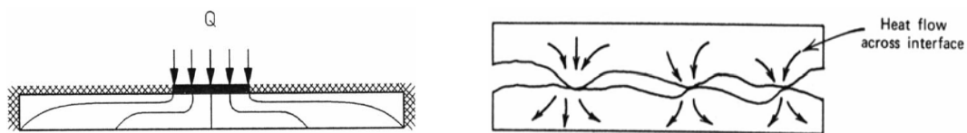
Figure 14. Spreading resistance and contact resistance schematics [54].
