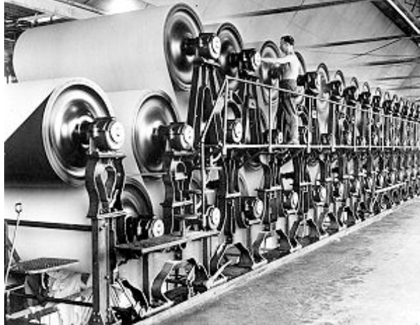
Figure 1.1: A classic example of a Fourdrinier machine
