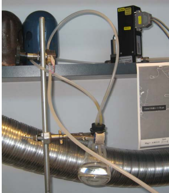
Figure 38. Bubbler apparatus used to introduce water vapor into the tube furnace.
