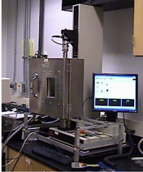
Figure 51. MTS Insight 2 electromechanical test system used to perform tensile tests.
