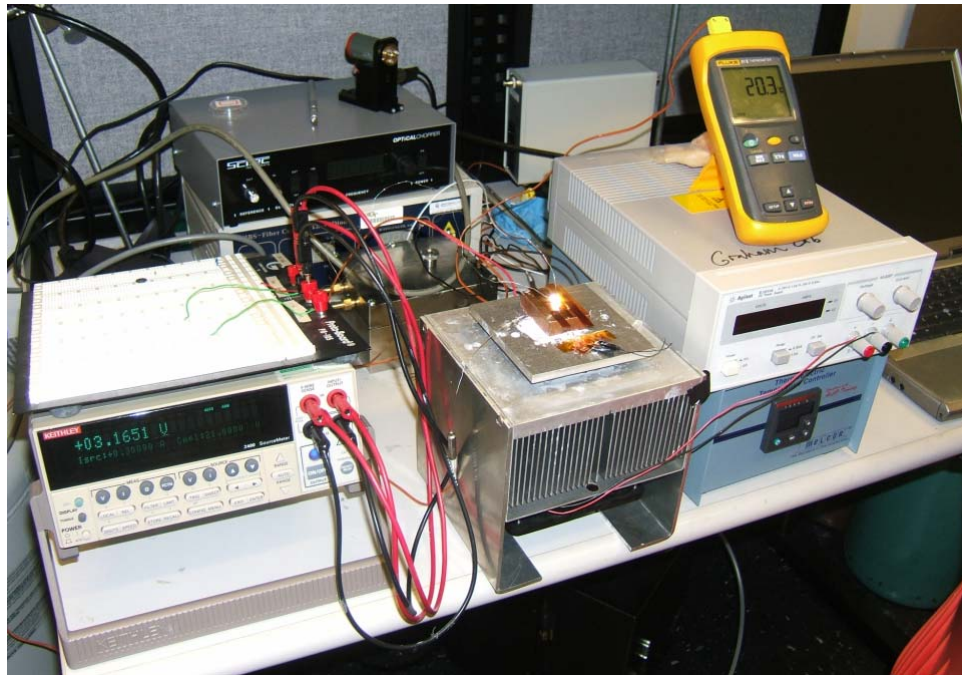
Figure 56. Experimental set up for LED thermal resistance measurements.
