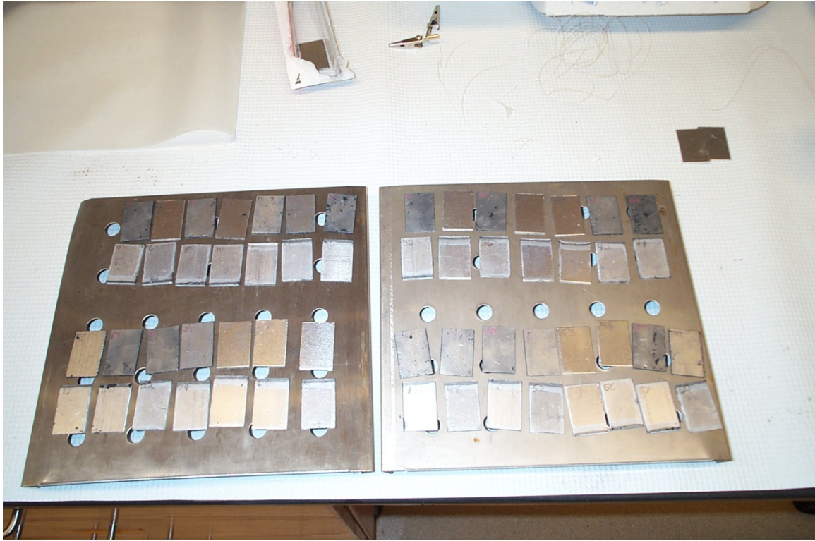
Figure 31: Specimens Contaminated with Graphite
