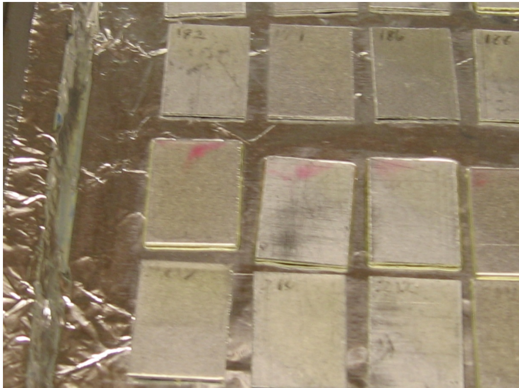
Figure 35: Motor Oil Contaminated Specimens
