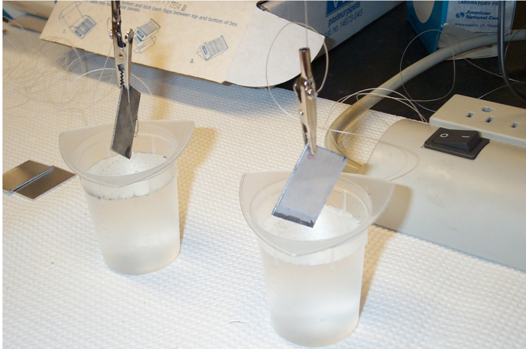
Figure 30: Specimens in Dipping Apparatus
