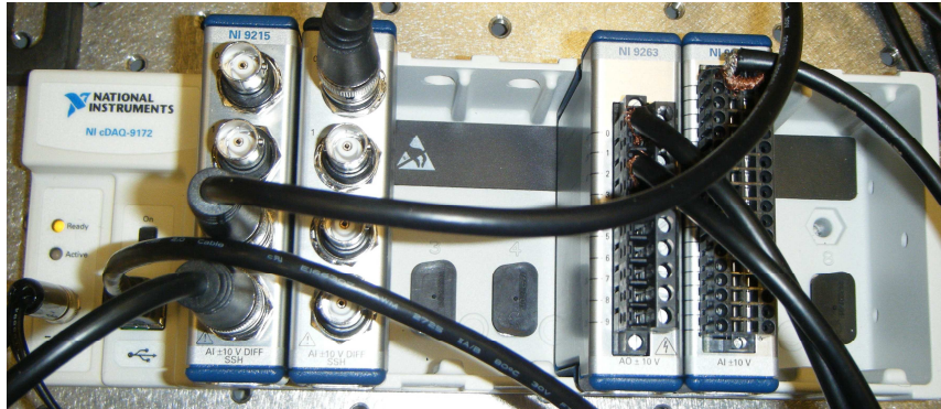
Figure 7: NI cDAQ-9172 CompactDAQ Chassis used to interface hardware with Labview software through analog input modules, an analog output module, and an analog trigger module.
