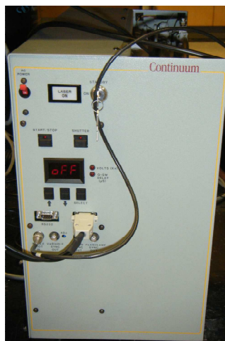
Figure 5: Power cooling unit and front control panel
