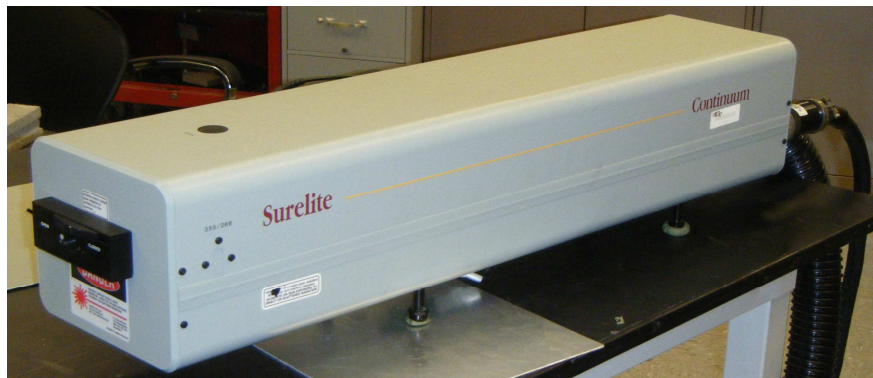
Figure 4: Surelite SL I-10 Nd:YAG high energy laser bench used as a point source excitation
