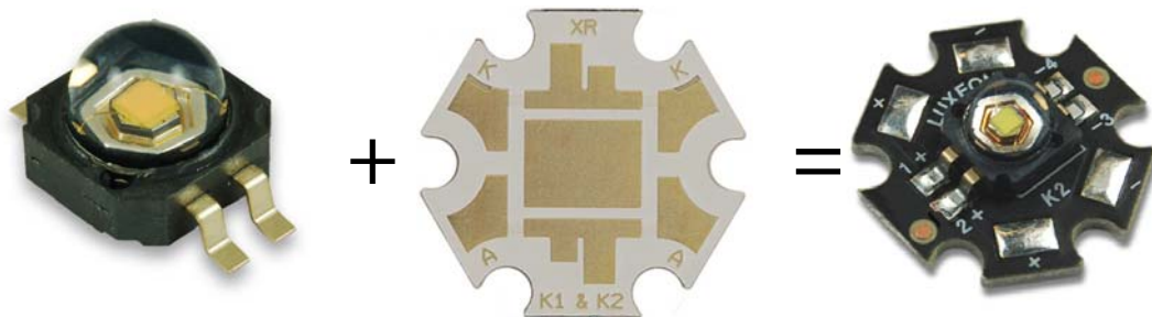
Figure 21. The heat slug package cannot be directly placed on a heat sink because the heat slug is not electrically isolated. IMS (MCPCB) makes the heat slug to be isolated and helps heat dissipation. The package shown in figure is LUXEON K2 Warm-White LEDs and Star Aluminum MCPCB [3].
