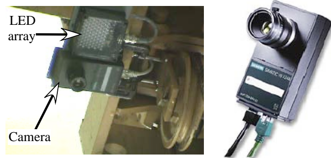
Fig 16. Trolley Mounted Camera - Closeup View (Photo on the Right Courtesy of Siemens)
