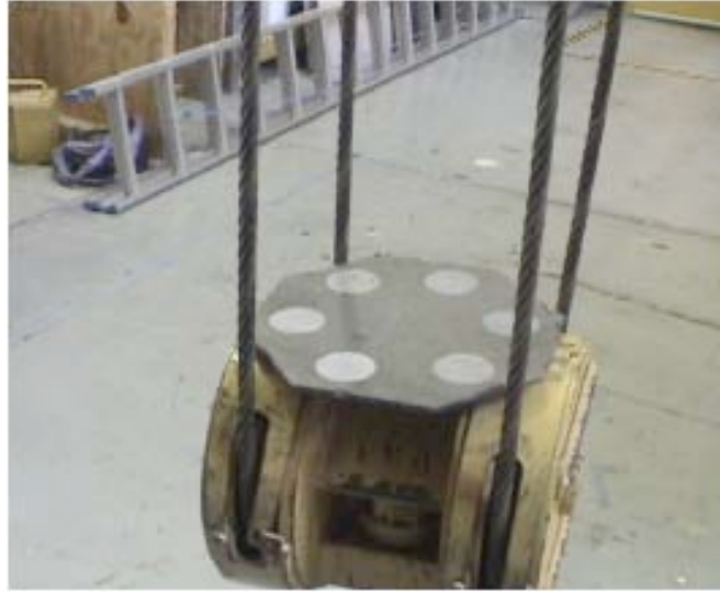
Fig 17. Reflective Material on the Hook
