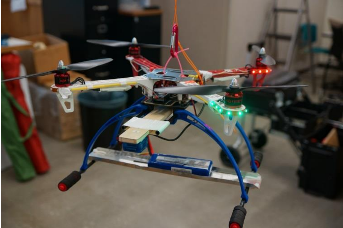
Figure 3.3: DJI F450 quadcopter platform with front/rear transmitters
