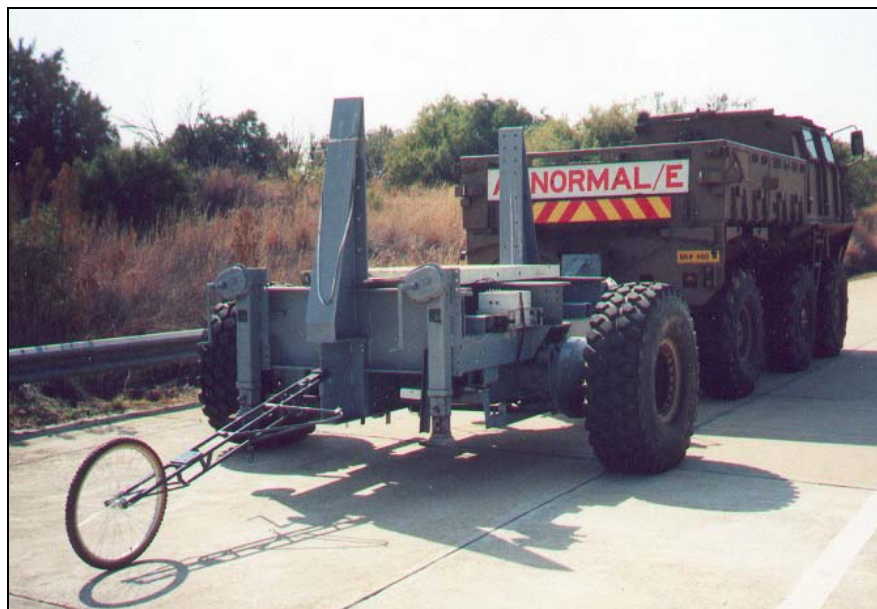
Figure 18 : Measuring tire data
