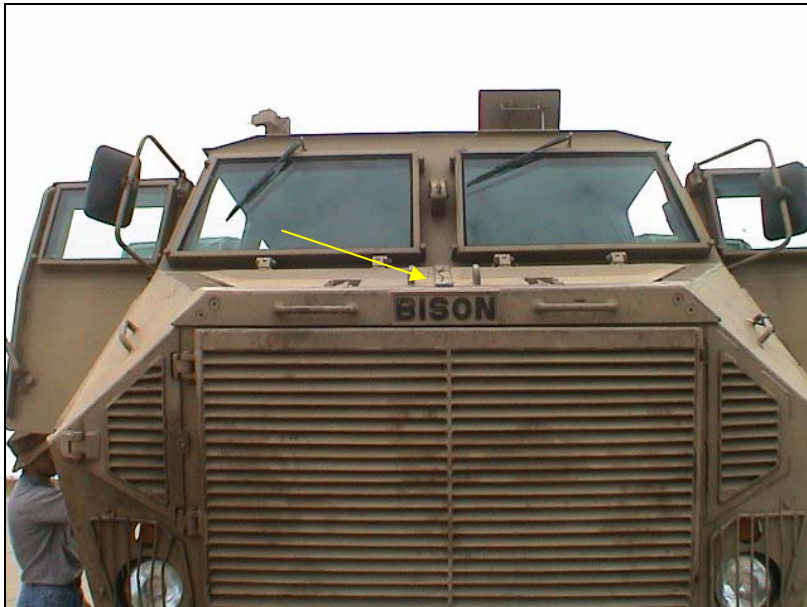
Figure 62 : Front GPS antenna position
