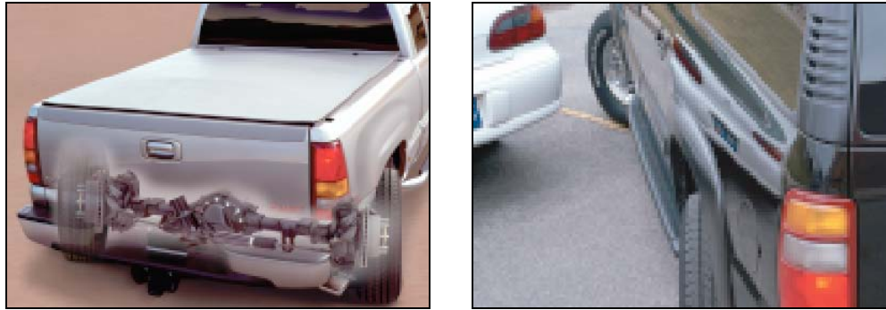
Figure 6 : EMAS automatic hydraulic steering [2]
