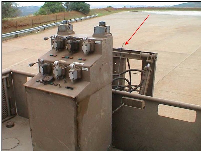
Figure 58 : Rear GPS antenna position
