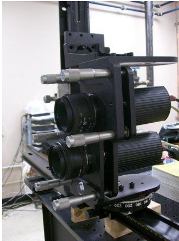
Figure 3-6 Two cameras configuration of 2D-PIV measurement for a large measurement domain
