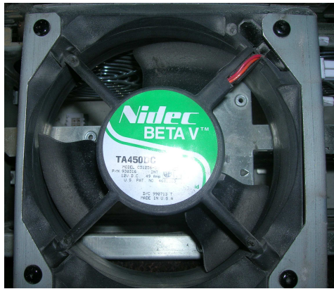
Figure A 13: Processor cooling fan in legacy server.
