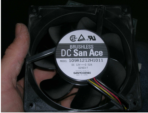
Figure A 12: Power supply cooling fan in legacy server.
