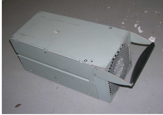
Figure A 15: Sample power supply for legacy server.
