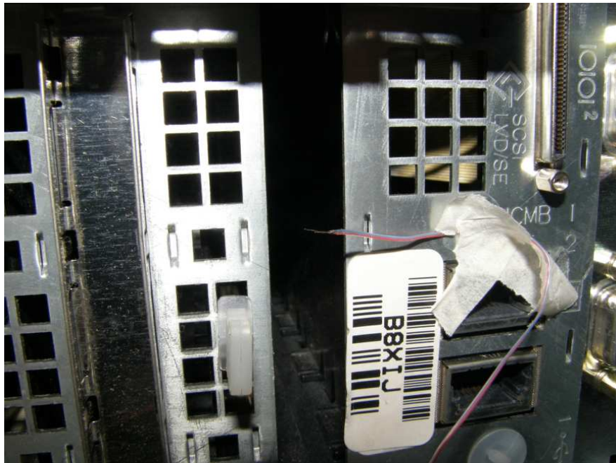
Figure A 34: Thermocouple placed at processor outlet of legacy server.
