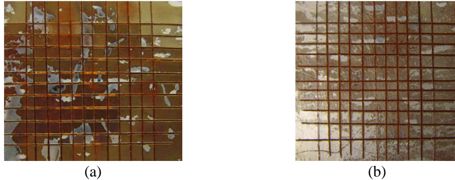
(a) (b) Figure 4.25 ASTM Tape test on NPS/Kapton HN adhesion (a) Ra=33nm (b) Ra=366nm
