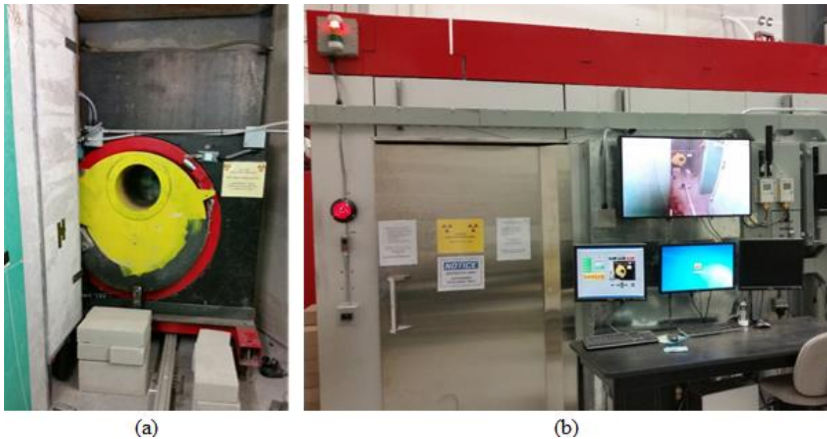
Figure 2.4 (a) The inside view and (b) the outside view of the imaging cave
