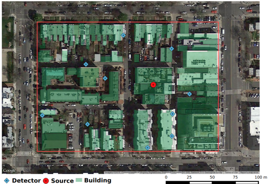
Figure 4.1: Satellite image of test location, with modeled geometry overlaid in green, as well as source (red) and detector (blue) locations.
