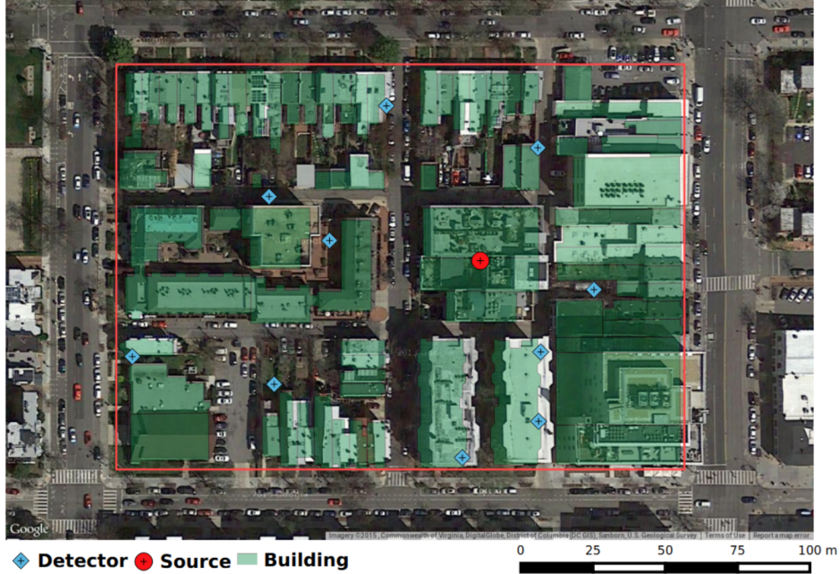
Figure 1.1: Example source localization problem, with a detector network distributed over a city block. We wish to determine the location of the source using only count rates measured by the detectors.
