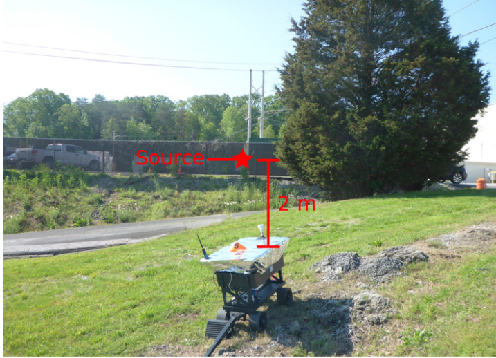
Figure 5.5: Elevation difference in experiment 2. The source is located just behind the fence visible in the background.
