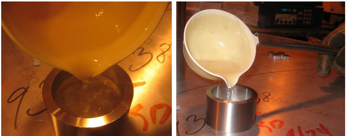
Figure A-2: The RbCl is heated to above its melting point and poured into a cast.
