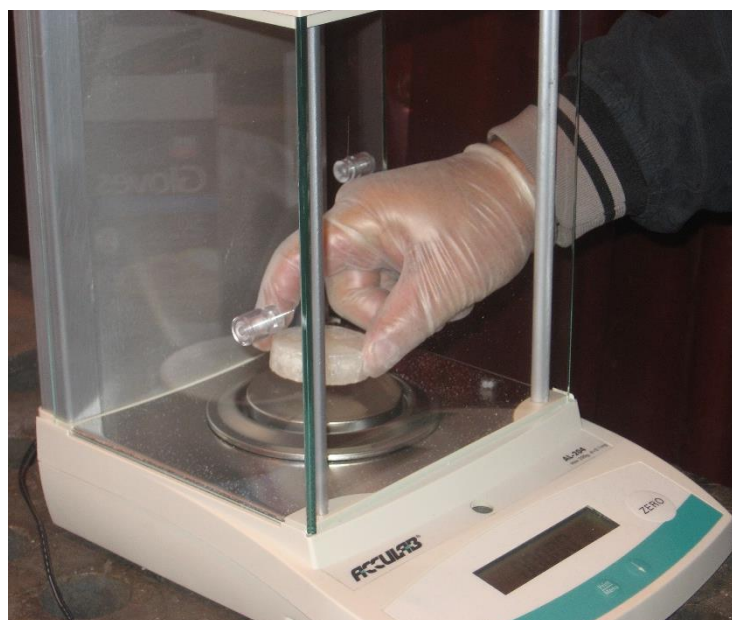
Figure A-4: The solid RbCl target puck is weighed and then ready to be encapsulated under vacuum.
