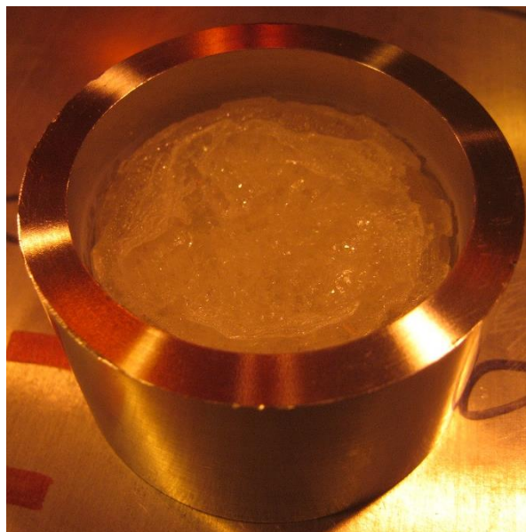
Figure A-3: The molten RbCl is left to solidify into a solid target puck.
