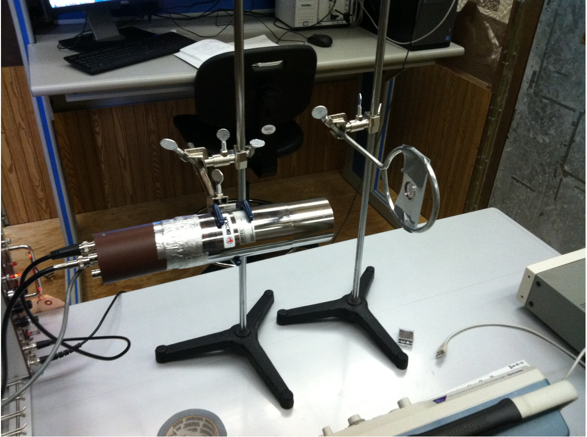
Figure C.2: NaI(Tl) with calibration source setup to collect PHS for validation of the fitting algorithms PHS.
