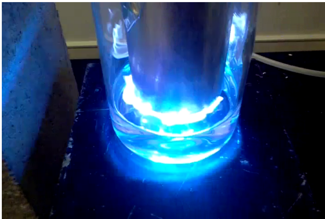
Figure 5.16 Photograph of 350 W “bright” argon discharge treating aqueous dioxane solution
