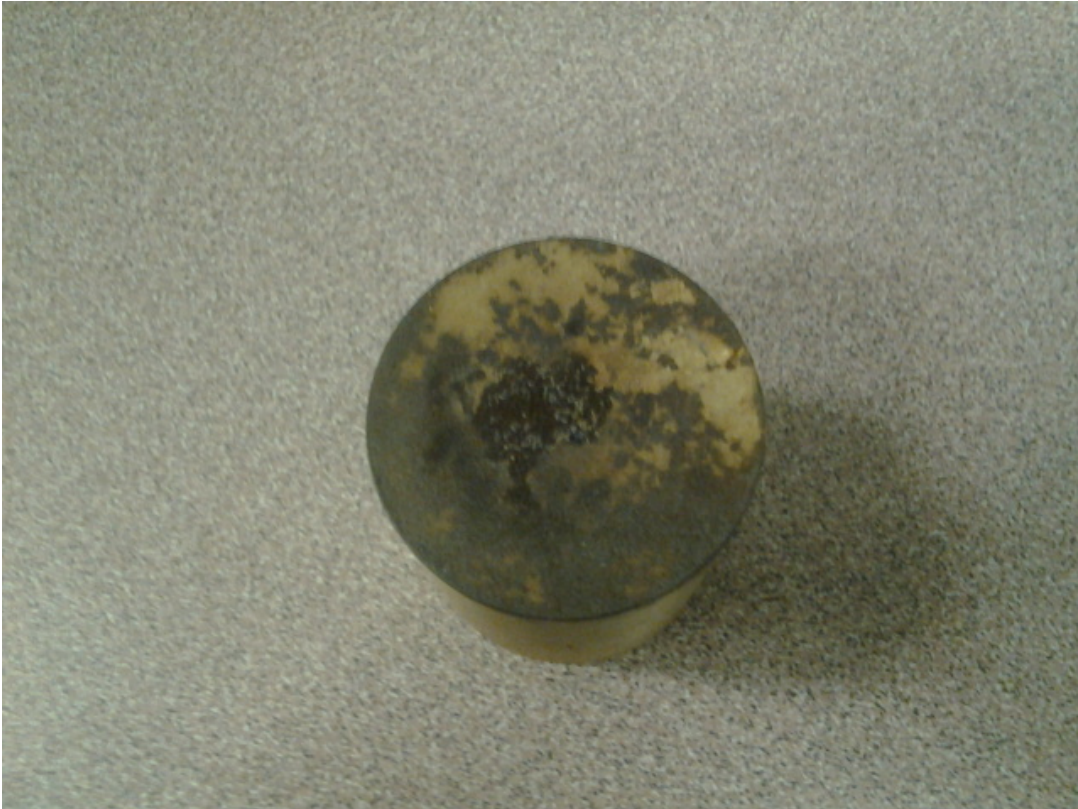
Figure 4.10 Image of brass electrode after plasma erosion
