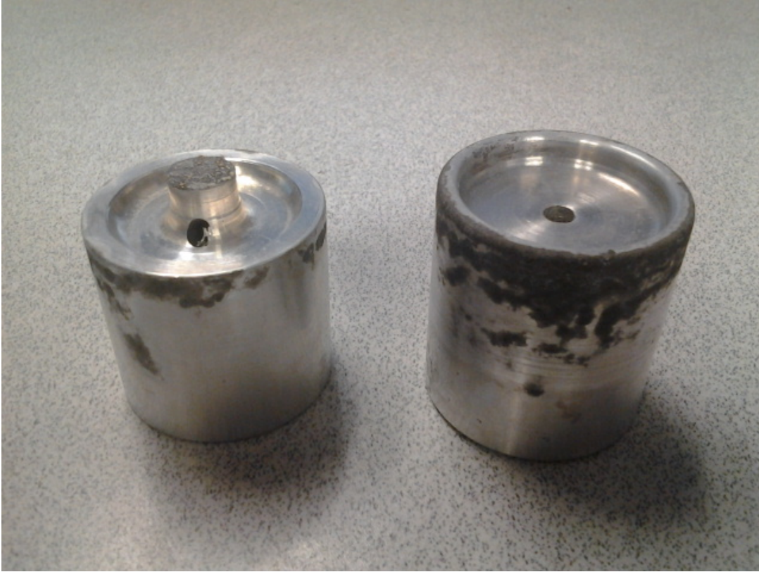
Figure 4.13 Image of the two versions of “water” electrodes. The “annular” version still allows a small metallic area of plasma contact. In the “pure” version, the plasma has no metallic content with the powered electrode. The powered surface is entirely composed of water.
