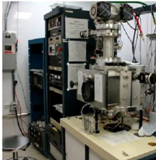
Figure 2.11: DC Sputtering used to Deposit Gold Contacts
