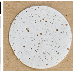
Pinholes through whole scaffold visible
