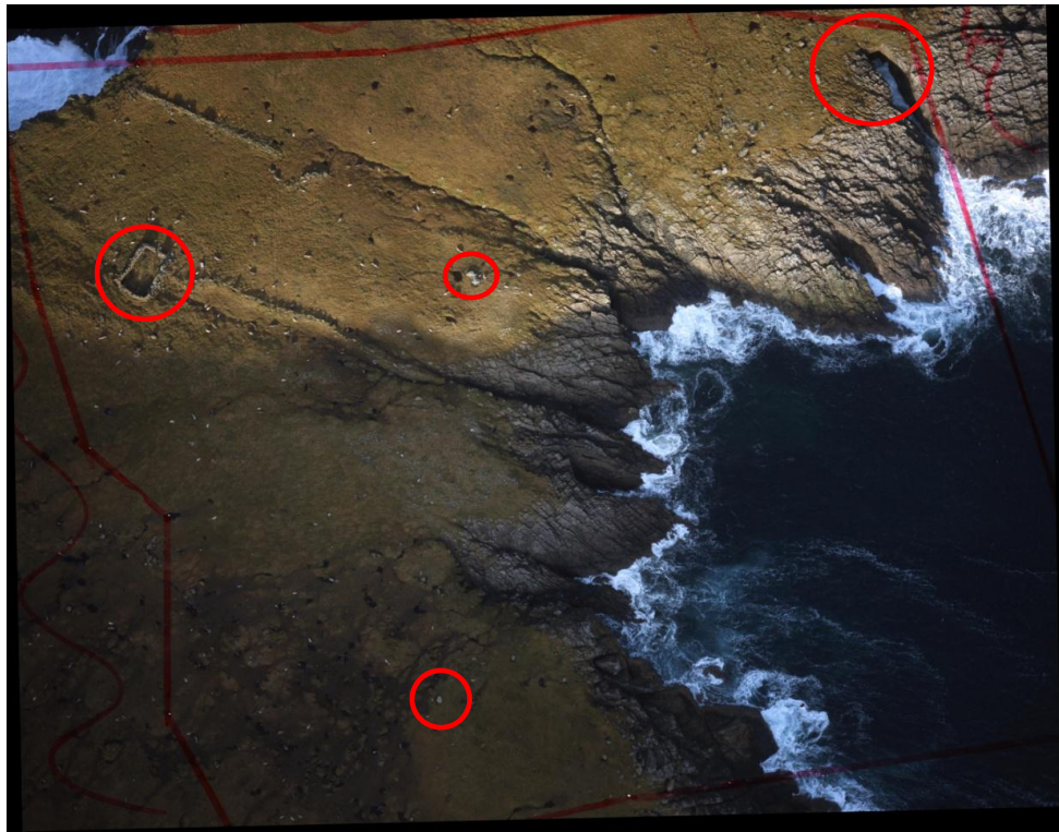
Figure 2.4: Example of an aerial photograph taken by SMRU for the annual pupping census. This photograph shows the main part of the SS, including several key features useful for georectifying the aerial photograph to real-world OS GB coordinates (circled in red).
