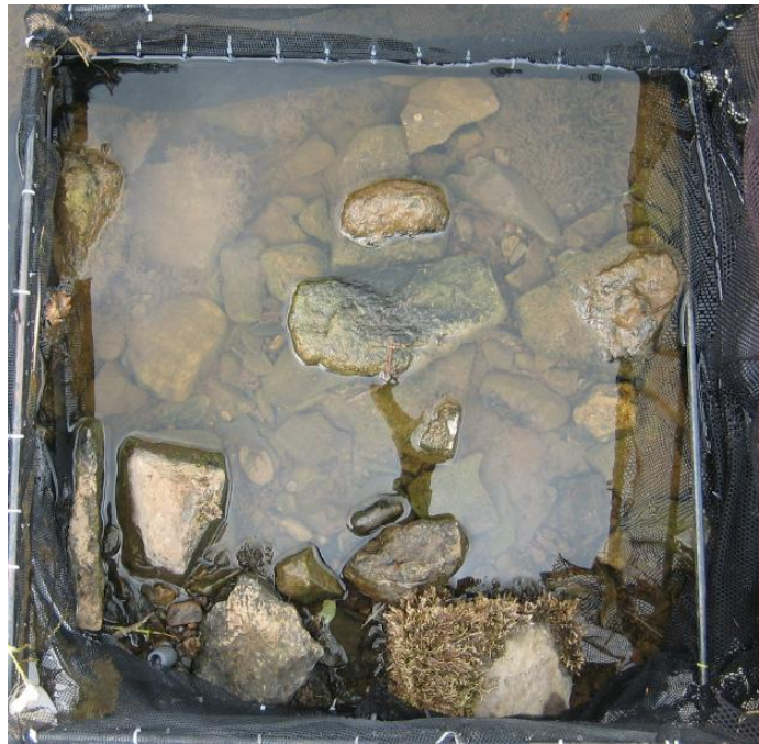
Figure 4.7 – Vertical photograph of a surber area used to measure grain size by manual photo-sieving
