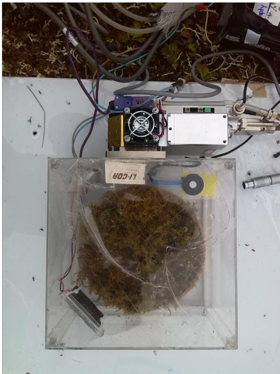
Figure 7: Hylocomium splendens inside the large chamber used for field experiments.
