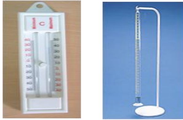
Fig. 3.3 Maximum and minimum thermometer and evaporimeter
