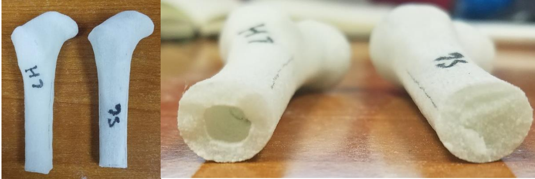
FIGURE 168. Sample fracture patterns of a hollow (labeled H7) and solid specimen (labeled S6) as a result of three-point bending loads. Posterior view (left) and transverse plane view (right).
