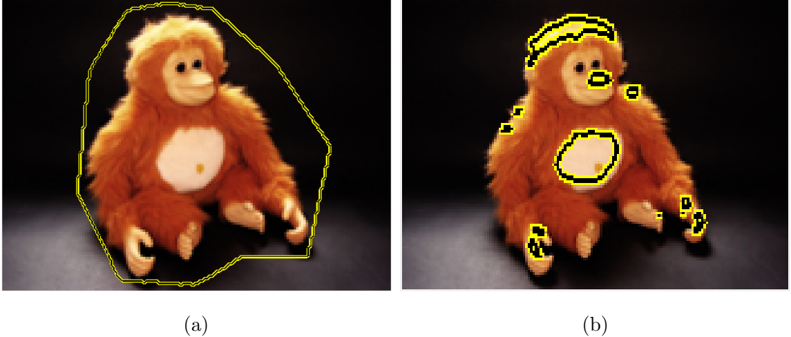
Figure 3.2: Incorrect segmentation using separation of means. (a) Original image and initial curve, and (b) final segmentation. The evolving curve is attracted to the brightest regions in the image.
