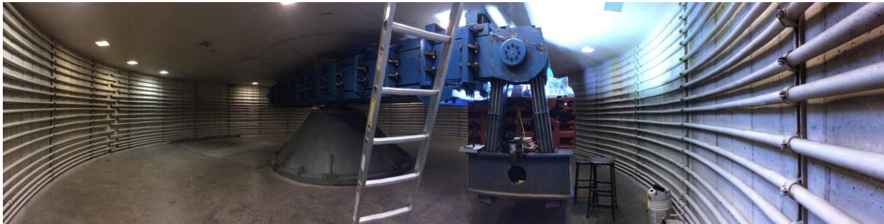
Figure 2.1. University of Colorado at Boulder 400 g-ton Geotechnical Centrifuge Facility with soil model installed on the payload platform.
