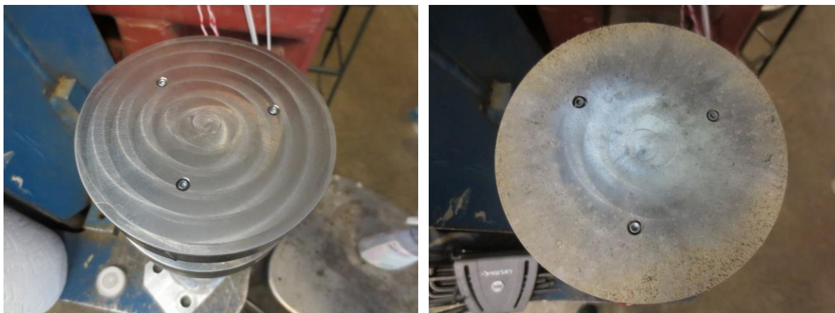
Figure 6.40. Target surface pre ( left ) and post ( right ) surface detonation of a 0.3 gram Detasheet charge at 10 g. Target positioned 5.1 cm aboveground. Note scorch marks and soil residue on target surface after detonation.
