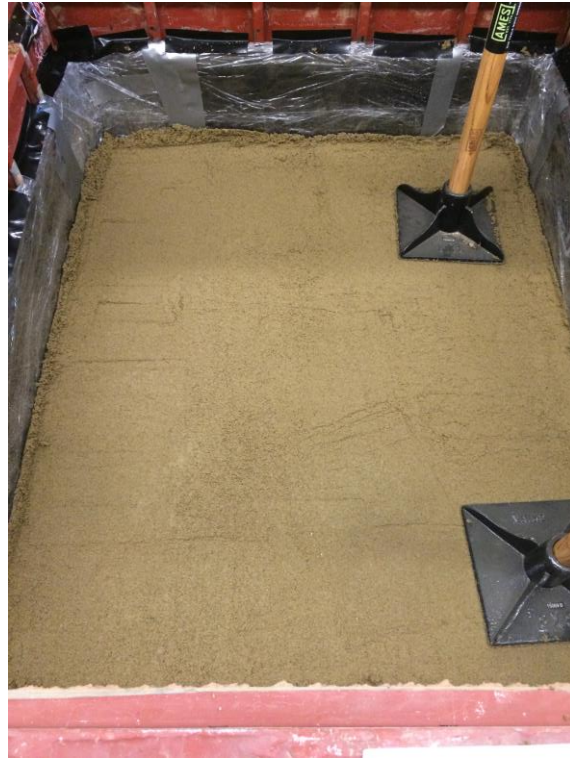
Figure 2.10. Prepared 80% sand and 20% clay model with 10% saturation (80s20c10w). Steel tampers compacted the centrifuge soil model.
