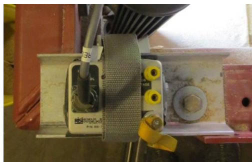
Figure 2.32 The Teledyne RISI FS-43 EBW ( left ) firing system Control unit and ( right ) Firing module (installed on centrifuge soil container).
