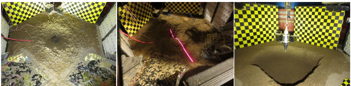
Figure 2.17. Test environment ( left ) post-detonation; ( middle ) laser profilometer scan of final crater surface; and ( right ) excavated testbed and overlying plumb bob readied for testing.
