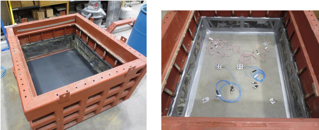
Figure 2.6. Elastomeric pads ( left ) and instrumented aluminum base plate ( right ).
