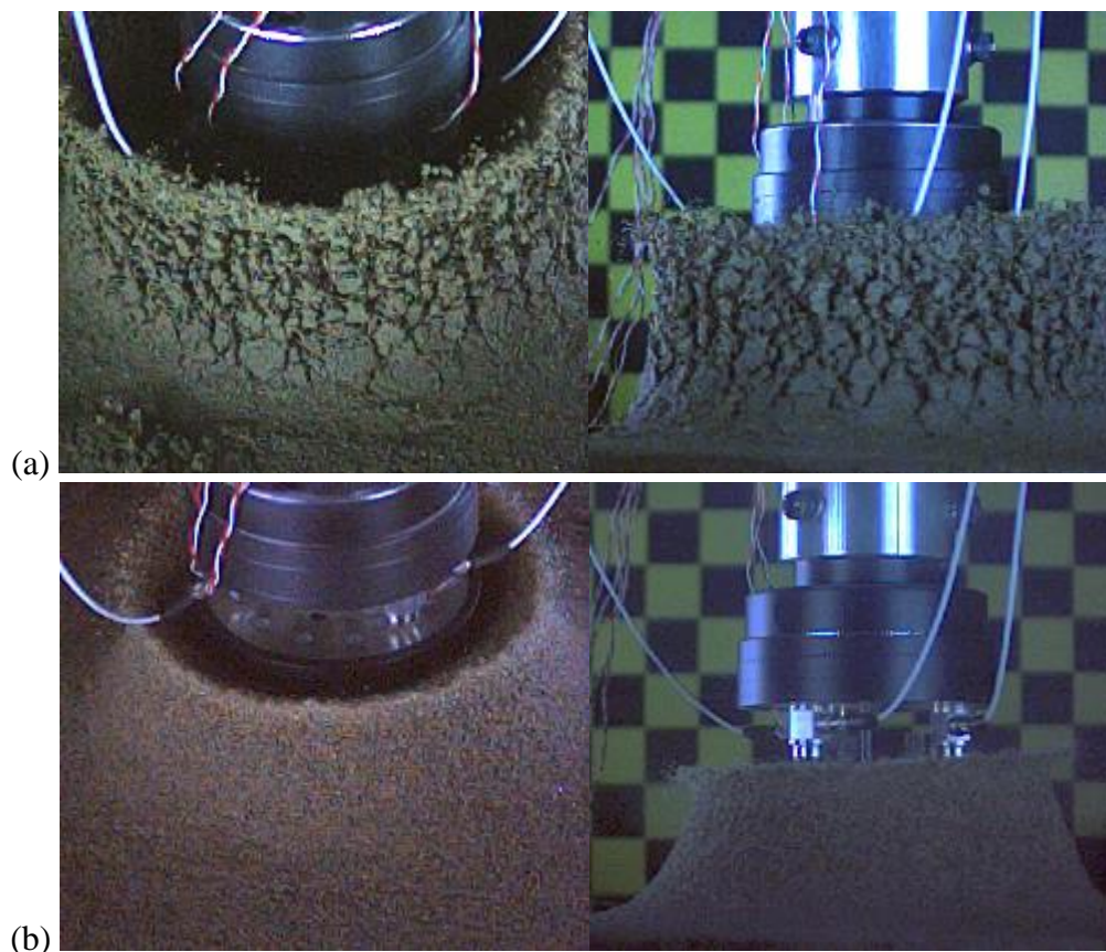
Figure 6.67. Comparison of the soil deformations for a 1.0 gram Detasheet charge buried 5.1 cm in (a) 80% sand, 20% clay with 10% water content (80s20c10w); (b) 10% saturated sand, and detonated at 10 g. Target positioned 5.1 cm aboveground. Frame time after detonation corresponds to negligible target response: (a) 4.80 ms; (b) 4.05 ms. Diagonal ( left ) and corresponding lateral ( right ) views provided. Fiducial background 2.2 cm square grid.
