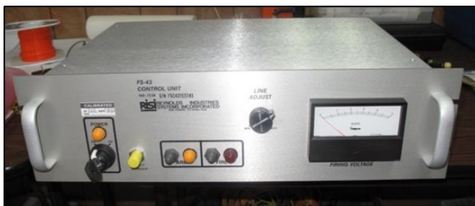
Figure 2.32 The Teledyne RISI FS-43 EBW ( left ) firing system Control unit and ( right ) Firing module (installed on centrifuge soil container).
