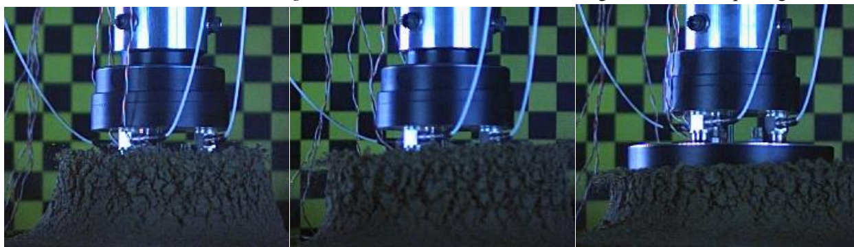
Figure 6.46. Comparisons of soil deformations for 1.0 gram Detasheet charge buried 5.1 cm in 80s20c10w and detonated at 10 g. Target positioned 5.1 cm aboveground. Time after detonation 3.61 ms for plate diameters: (left) 10.16 cm; (middle) 12.19 cm; (right) 15.24 cm. Fiducial background 2.2 cm square grid.
